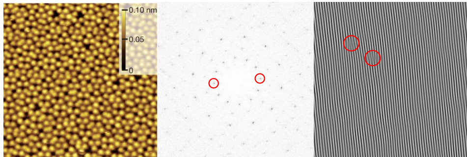
Fig.1: (a) Example of a segment from an STM image of a dodecagonal quasicrystal, of a Ba-Ti-O-derived thin film phase on Pt(111) [1], showing several dislocations. (b) Fourier transform of the atomic positions of an STM image from the same dataset, with the central peak blocked. A pair of Bragg peaks, associated with one of the basis vectors and its negative, is marked in red. (c) The corresponding section of the inverse Fourier transform of the filtered Bragg peaks marked in (b) with red circles marking the positions of two dislocations.
